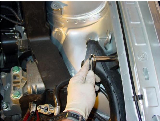
12....remove the ducting (nut will be reused)
