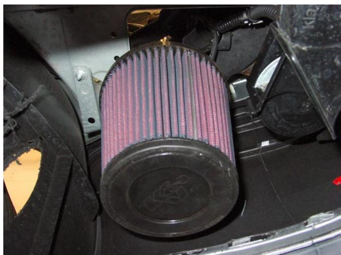
20. Install the air filter from underneath
