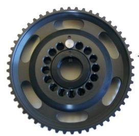
note the reference marks: this sprocket is shown with the lock pin in its stock (zerochange) position.
