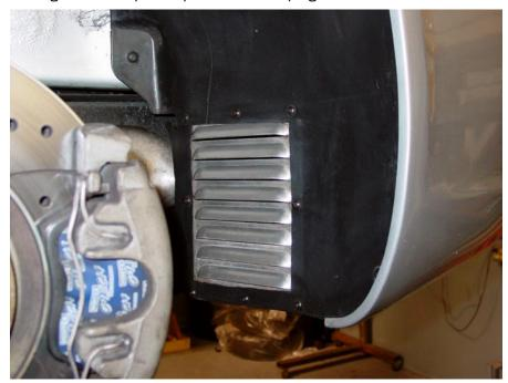
3) Position the template on the liner about an inch up from the bottom and an inch and a half out from the inner edge. Observe the webbing on the intercooler-side of the fender liner. You may want to adjust the position of the template to find the "sweet spot" relative to the webs, so as to avoid interference with the mounting screws.
