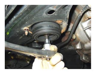
Next, using an 8mm hex (Allen®) wrench, remove the bottom center bolt as shown (above right) and take out the lower bushing.
