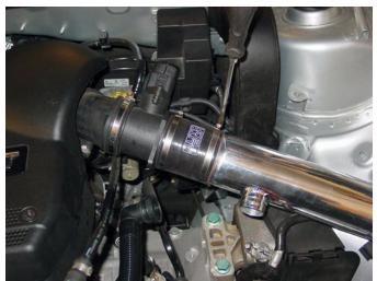
19. Install the nut on the flange of the tube
