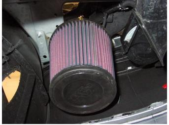
20. Install the air filter from underneath
