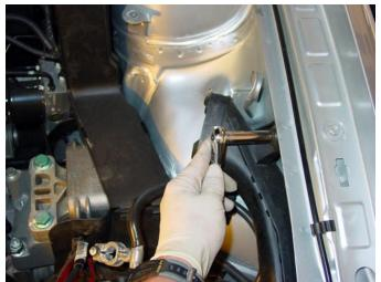
12. ...remove the ducting (nut will be reused)
