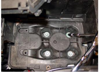
7. Remove the four bolts holding down the battery tray
