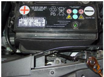
24. Re-attach the battery hold down
