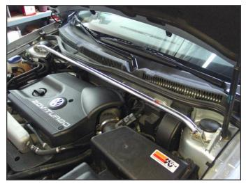
11. Using a 9/16" wrench, "snug" the jam nut against the crosstube (fig 9). Torque is approx 8 ft lbs.
