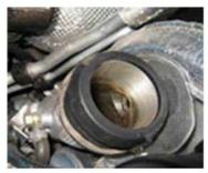
Using channel lock pliers release tension on the clamp that connects the turbo inlet pipe to the turbo. Then remove the turbo inlet pipe. There is a rubber grommet inside the inlet pipe that will sometimes remain behind, that will need to be removed too, as seen in the picture.
